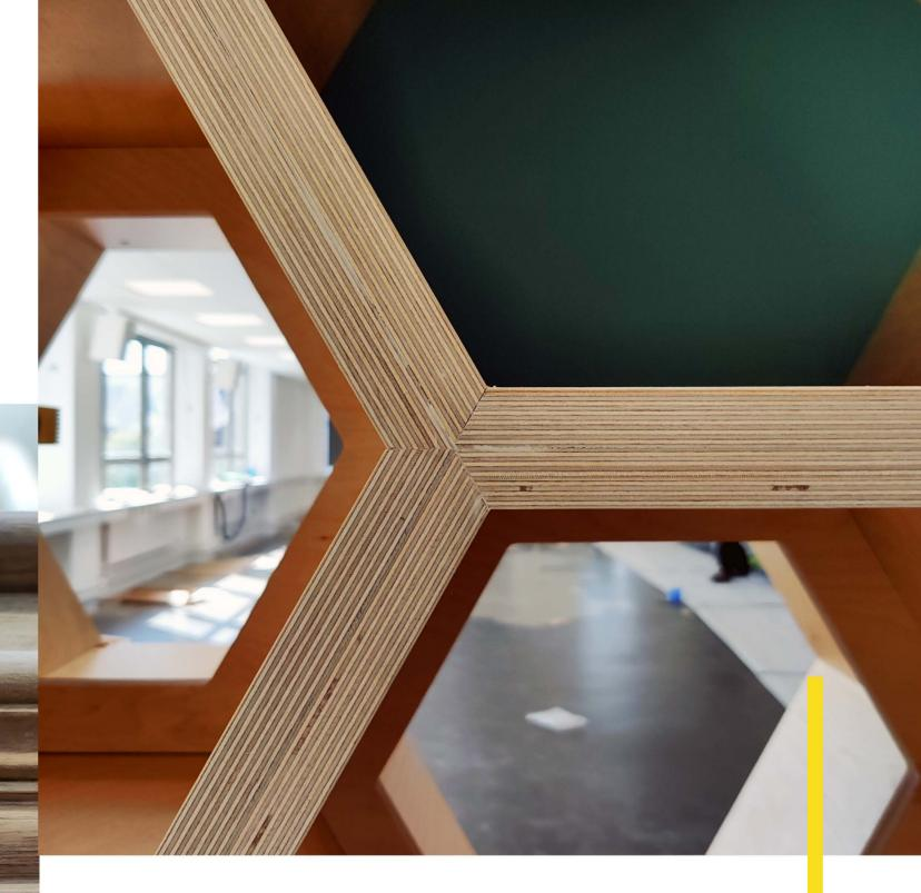
Shown here in seamlessly jointed birch plywood, this shelving unit was handmade in our Bristol workshop as part of a larger commercial project for Bristol University. This project was crafted using our dimension saw and bonded in a clamp jig we constructed just for this single project.
